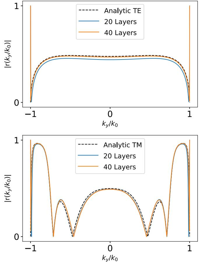
**Fig. 7.** The reflection coefficients for the TE (top) and TM (bottom) case are given for the multilayer approximations to the continuous profiles shown in Figure 1. The reflection coefficients are not affected significantly, there remaining a range of angles at almost grazing where the reflectivity is close to zero.
