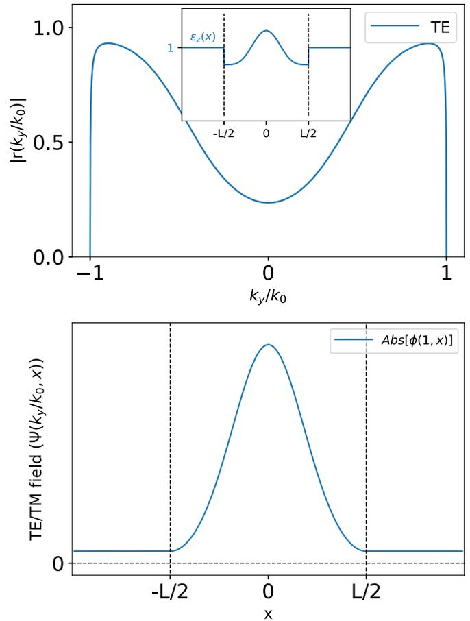
**Fig. 5.** A profile  $\varepsilon_z(x)$  (inset) is designed to specifically have a large discontinuity at the boundary between the material and the vacuum. As a result, the reflectivity (top) exhibits large reflection at angles close to grazing but still goes to zero at grazing. The field profile (bottom) is given to show that the system still supports a HBS.
