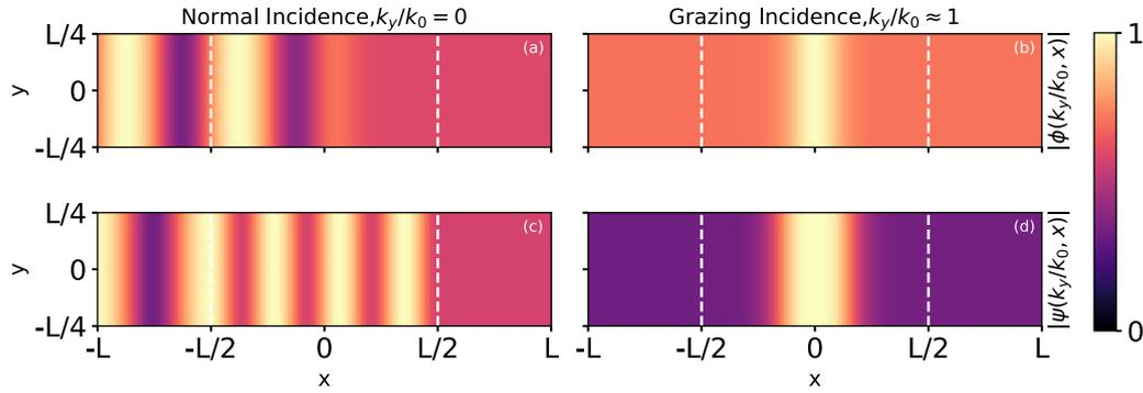
**Fig. 2.** The field distributions (for the device in Fig. 1),  $|\phi|$  of a TE wave incident at normal (a) and grazing ( $\theta = 89^\circ$ ) (b). Similarly for the TM case,  $|\psi|$  for normal (c) and grazing ( $\theta = 89^\circ$ ) (d). At normal incidence, the absolute value of the field is not constant on the left, indicating there is reflection, whereas for grazing, the equal field amplitude on the two sides of the profile shows that there is no reflection.
