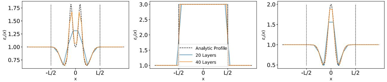
**Fig. 6.** The distribution for the  $x$  (left),  $y$  (middle) and  $z$ - (right) diagonal components of the permittivity tensor for the stacked structures of 20 and 40 layers compared to the analytic profiles (black dashed).
