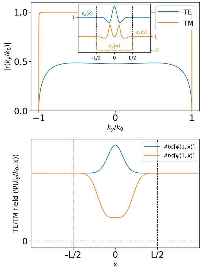
**Fig. 3.** A hyperbolic material with constant  $\epsilon_y = -3$ , and  $\epsilon_x, \epsilon_z$  staying the same as in Figure 1. The top panel shows that although the TM case has almost complete reflection, at grazing incidence the profile of  $\epsilon_x(x)$  ensures there is no reflection at grazing.
