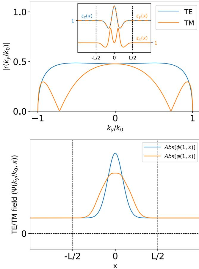
**Figure 4.** A uniaxial anisotropic material is defined as one whose  $\varepsilon_y(x) = \varepsilon_z(x) \neq \varepsilon_x(x)$ . The two permittivities  $\varepsilon_z(x)$ ,  $\varepsilon_x(x)$  (inset) ( $\beta(x)$  and  $\alpha(x)$ ) are the same as in Fig. 1) are designed to ensure that the material exhibits zero reflection at grazing (top) as a result of the material supporting a HBS for both polarisations at grazing incidence (bottom).
