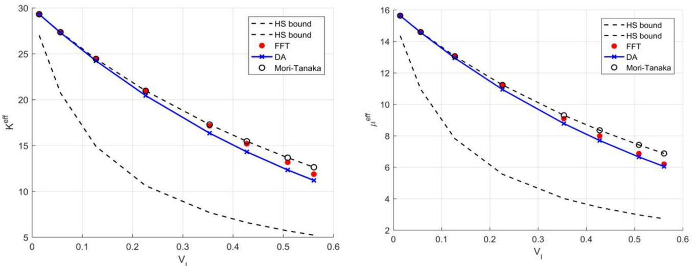
**Fig. 3.** Elastic bulk (left) and shear modulus (right) of three-phase composites with the case (B).
