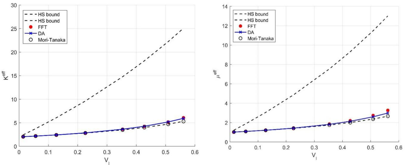
**Fig. 2.** Elastic bulk (left) and shear modulus (right) of three-phase composites with the case (A).
