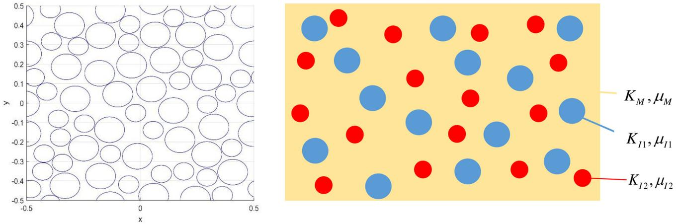
**Fig. 1.** Unit cell containing 60 circle-inclusion randomly placed (left), three phase model of composite with two different circles inclusion (right).
