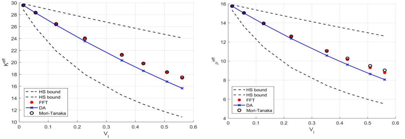
**Fig. 4.** Elastic bulk (left) and shear modulus (right) of three-phase composites with the case (C).
