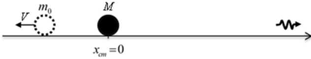
Fig. 2. The atom emits a photon reducing the mass and recoils to the left.
